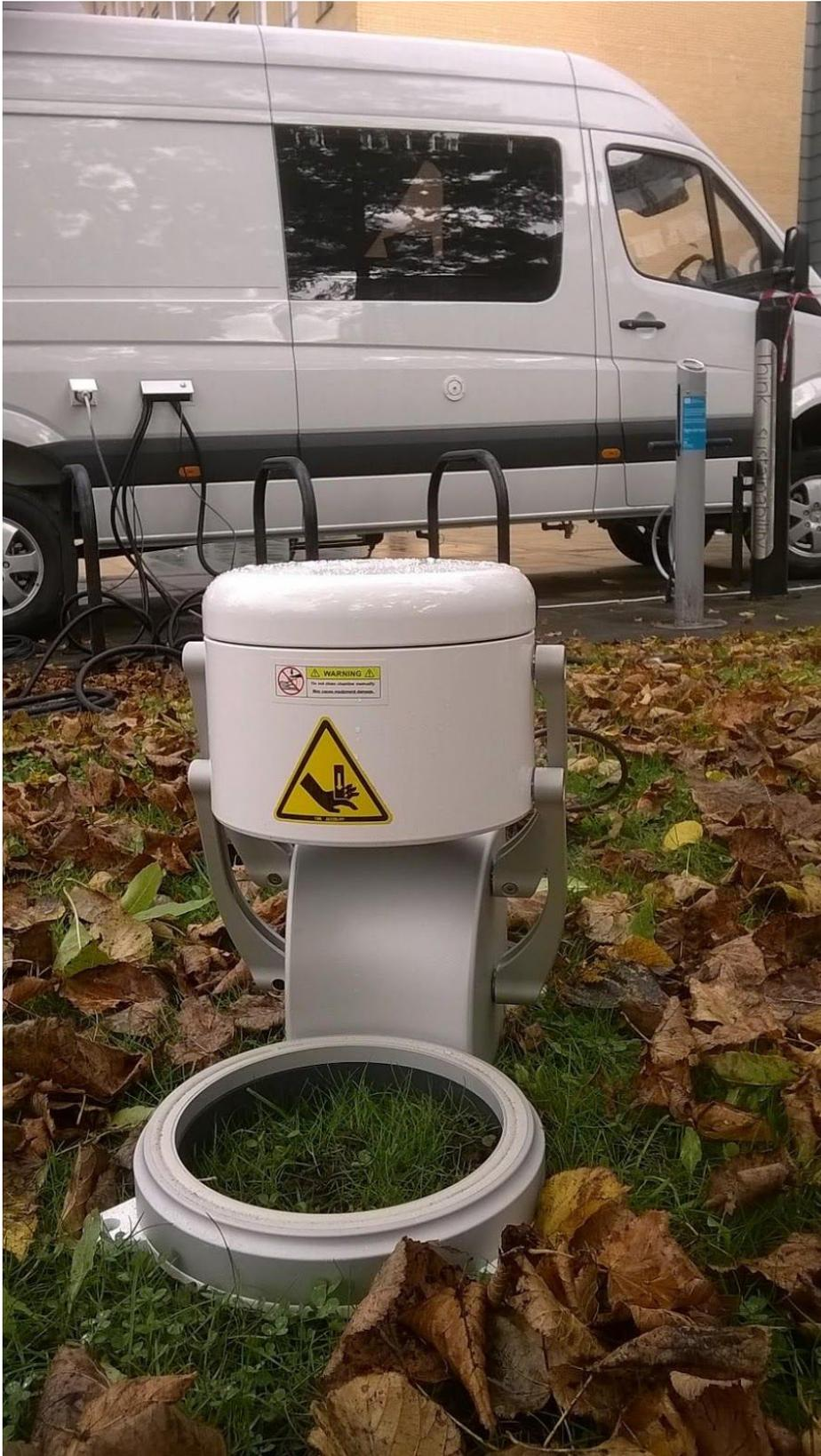
One of the 12 automated soil gas flux chambers to allow continuous monitoring of greenhouse gases
