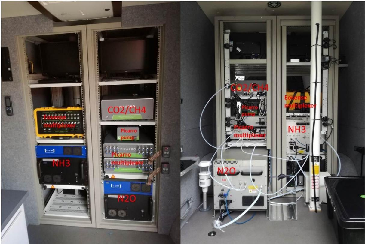
Internal arrangement of instrumentation showing cutting-edge laser absorption spectrometers for real-time measurement of isotope ratios in gases
